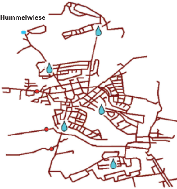
▲ Fig. 3: Methodology and result of a simulation with LeakControl position optimizer in Stuttgart
