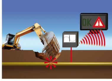
How the new smart CCP system works
