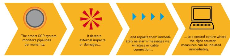
What's more, the smart CCP system now allows network operators to implement a remote CCP monitoring system according to DVGW GW 16, Category 2c on many pipelines for which this is impossible with the available conventional technology.
